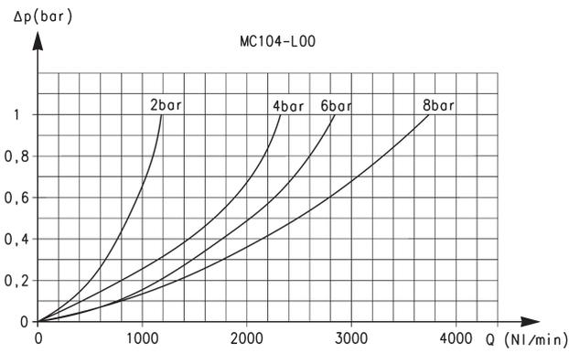
Flow diagram for model: MC104-L00
