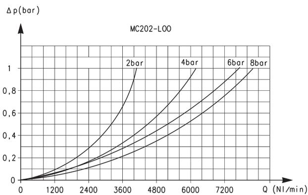
Flow diagram for model: MC202-L00
