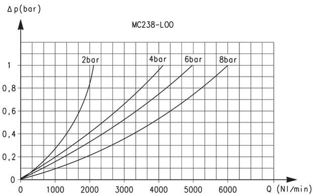
Flow diagram for model: MC238-L00
