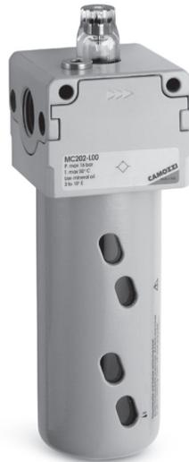
Series MC lubricators are available with ports G1/4, G3/8 and G1/2. The bowls of these lubricators are made of metal and are equipped with a transparent viewer. The oil flow can be monitored through the small transparent cap and regulated by means of the proper adjusting screw.
