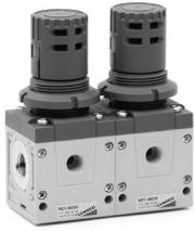
With the Manifold version it is possible to realize a battery of regulators which are fed by a single source of inlet pressure. Each regulator can be set up at any pressure (lower than the inlet pressure). The front or rear connection of each regulator allows to draw air at the pressure value set on the regulator itself.
